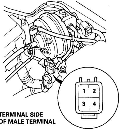
2. Check for resistance between the terminals according to the table.
